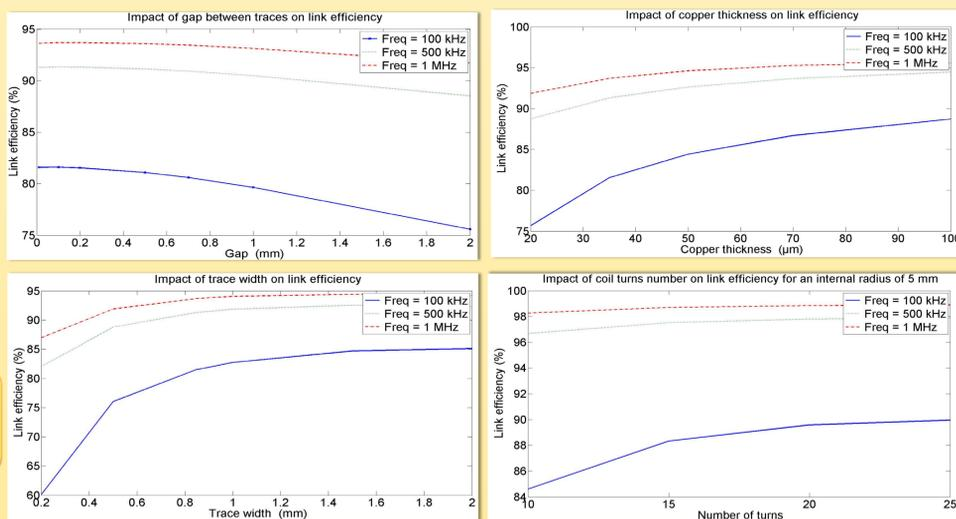
Fig. 5: Coil parametric study on Gap (top left), copper thickness (top right), trace width (bottom left) & turns number with Rin=5mm (bottom right). All parameters except the analyzed one were constant and identical to basis coil's ones.
