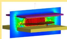
The maximum link efficiency is obtained for  $d=2\text{mm}$ ,  $\mu_r > 100$  and  $\text{RAR} > 1$ . By using a ferrite the link efficiency was improved with 4% at 100kHz.
